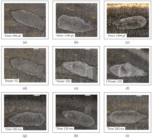
*Figure 9*. Effect of parameter changes on the central unbonded area of the joint: (a)–(c) Fixed: bond power: 80, bond time: 130 ms, bond force was increased; (d)–(f) Fixed: bond force 800 gf, bond time 130 ms, bond power was increased; (g)–(i) Fixed: bond force: 800 gf, bond power: 80, bond time was increased
