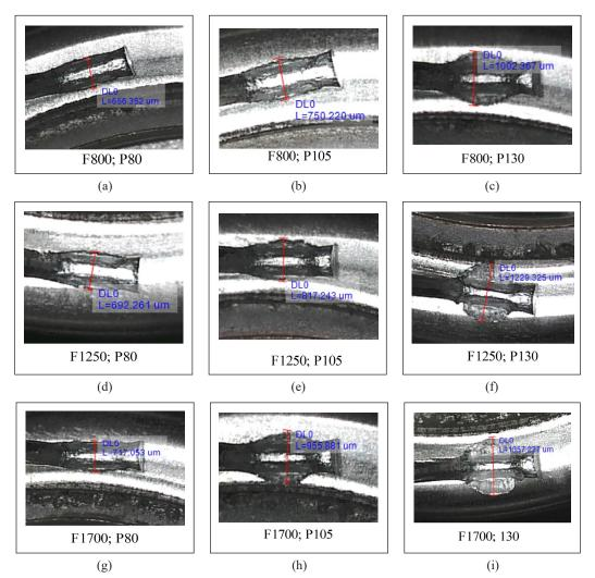
*Figure 11.* Joint width profile under different parameters: (a)–(c) Fixed: bond force: 800, bond power was increased; (d)–(f) Fixed: bond force 1250 gf, bond power was increased; (g)–(i) Fixed: bond force: 1700 gf, bond power was increased
