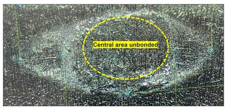
Figure 1. Morphology of the central unbonded area
