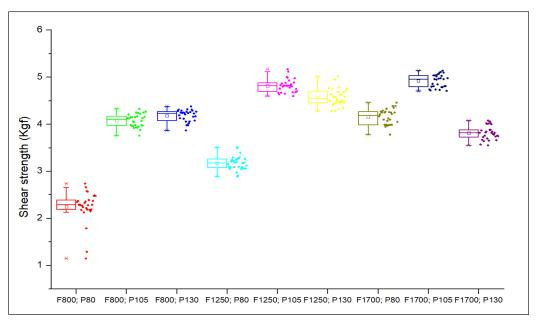
Figure 10. Box plot of shear strength under different parameters
