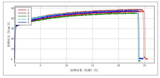
Figure 6. Stress-strain curve of Al wire
