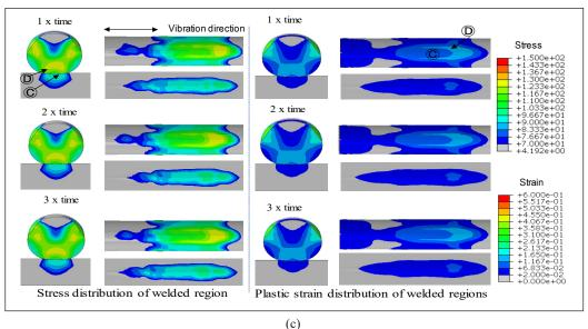
Figure  $\delta$  (continue). Simulation result under different parameters: (b) effect by bond power; (c) effect by bond time
