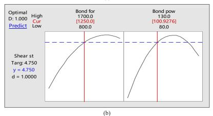
*Figure 12.* (a) Contour plot of shear strength vs bond power, bond force; (b) The optimal parameters obtained by the response optimizer
