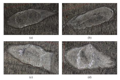
*Figure 3*. Morphology of weak bonded samples: (a) No. 1 unbonded; bond force 800 gf, bond time 130 ms, bond power 60; (b) No. 2 strength < 300 gf; bond force 1400 gf, bond time 130 ms, bond power 80; No. 3 strength < 800 gf; bond force 800 gf, bond time 130 ms, bond power 100; (d) No. 4 strength < 1500 gf); bond force 800 gf, bond time 130 ms, bond power 130
